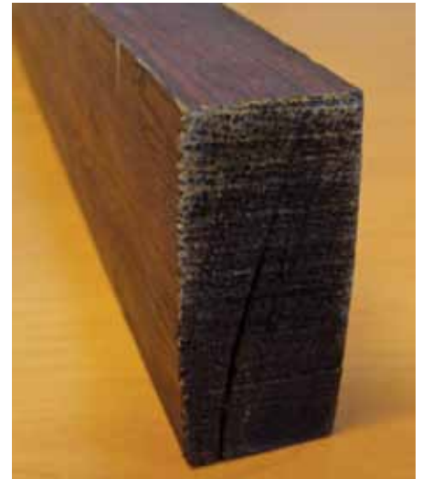
Figure 1. Stave of 18mm stave used for wine ageing and then cut lengthwise.
